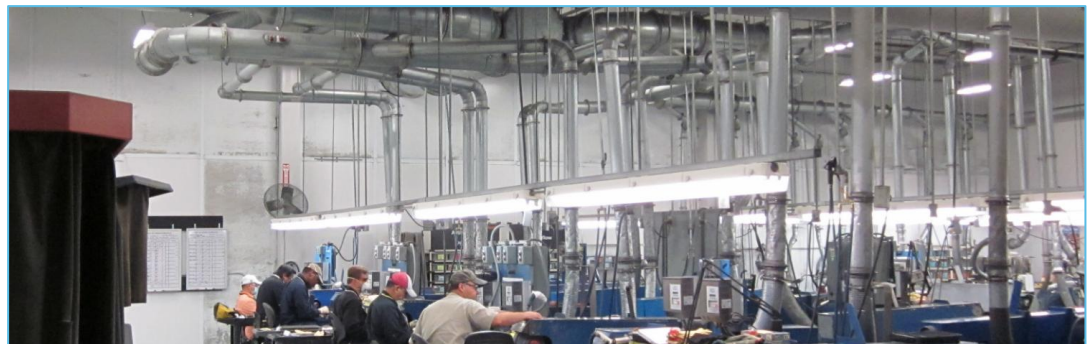
Portable weld fume collectors are specifically designed to capture and contain submicron weld fume from multiple locations within a facility.
